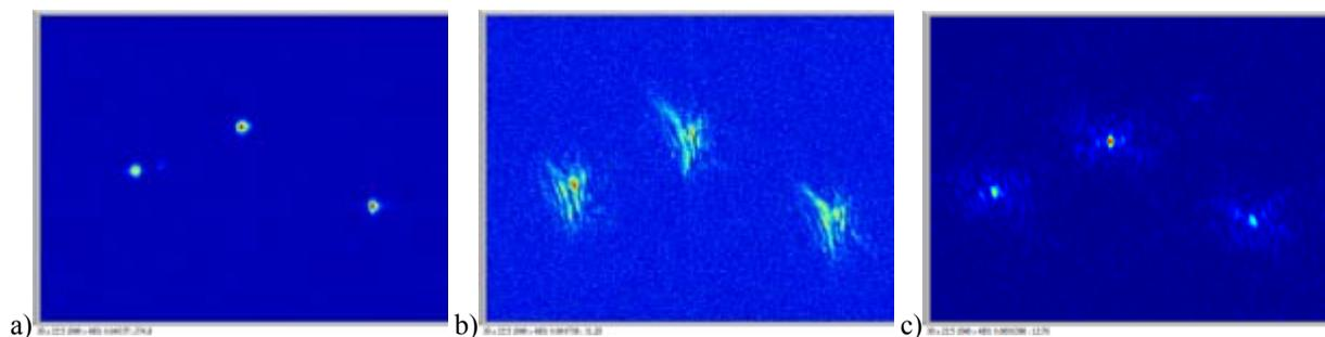
**Fig. 1.** Aberration compensation and adaptive optics by SIDH, demonstrated using LEDs: a) SIDH holographic image without phase aberrator; b) image with an aberrator in place; c) aberration-compensated by correlation with SIDH hologram of a guide star.
